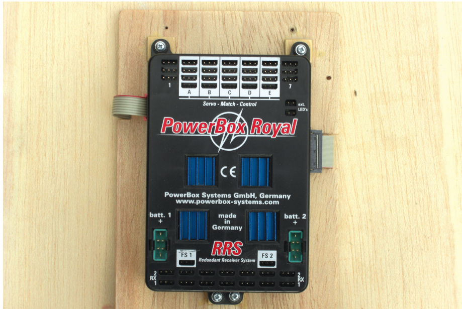
Royal unit mounted using the supplied rubber grommets and with leads from the LCD display and SensorSwitch connected
